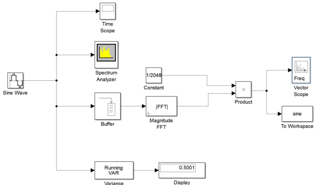
Figure 2: Simulink® Model of a Sinusoidal Wave for determining the Spectrum and Power Spectrum
